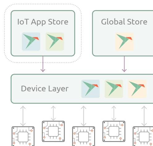
Diagram showing a typical store connection to a number of devices. Cherry pick the software you want your devices to see: in this diagram, two applications from the IoT App Store and one application from the global store have been selected for the device layer. These are the three applications that the devices will see and use.
